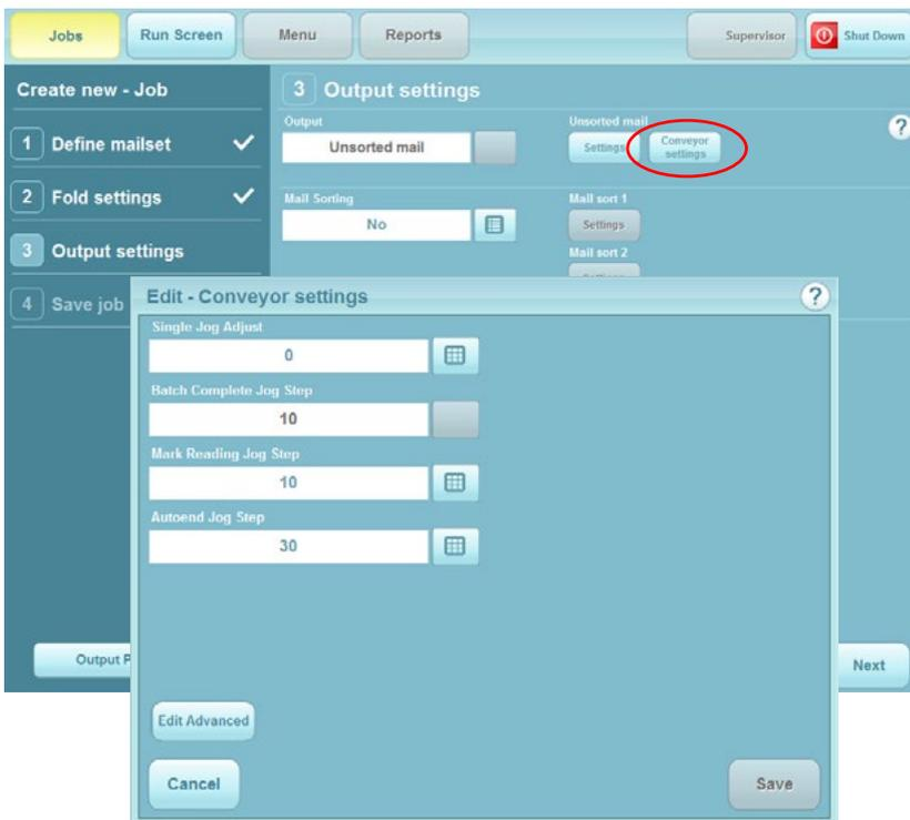
**3** If a conveyor is fitted, select **Conveyor Settings** to adjust the Jog functions as follows:
